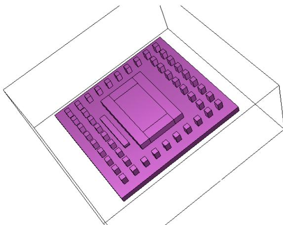
**Figure 5:** The component model from bottom side including the solder balls, driver, VCSEL, the Photo-Diodes arrays with the encapsulation material (the PCB is hidden).
