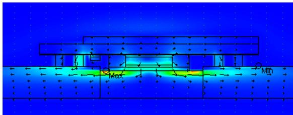
Figure 14: case-3 - Heat flux map from the VCSEL and the Photo-Diodes arrays to the PCB
