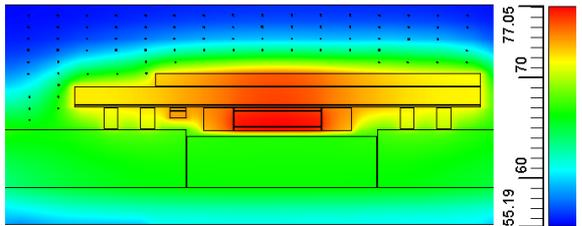
Figure 13: case-4 - temperature distribution at a central cross section
