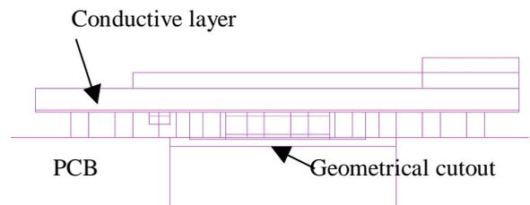
**Figure 7:** The component model cross section at a wire frame view.
