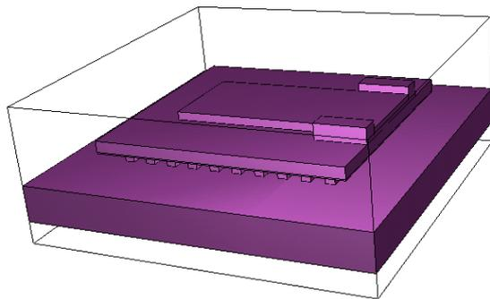
**Figure 4:** The component sub-modeling region Includes part of the PCB and the details component
