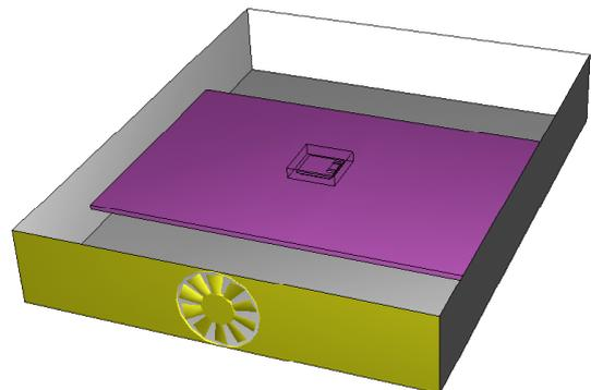
**Figure 2:** The JEDEC defined enclosure including the component sub model volume
