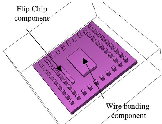
**Figure 6:** The component model from bottom side including the solder balls, driver, VCSEL, the Photo-Diodes arrays, without the encapsulation material (the PCB is hidden).
