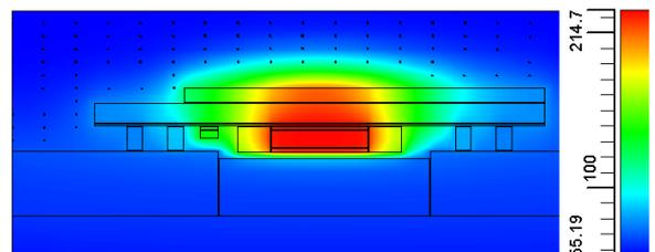
Figure 10: case-1 - temperature distribution at a central cross section
