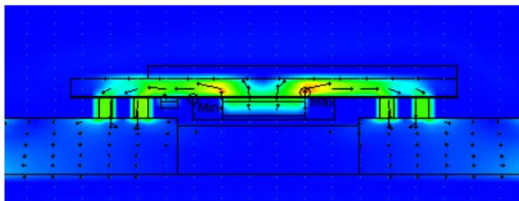
Figure 15: case-4 - Heat flux map from the VCSEL and the Photo-Diodes arrays to the PCB
