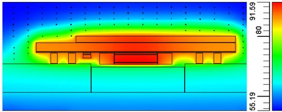
Figure 11: case-2 - temperature distribution at a central cross section
