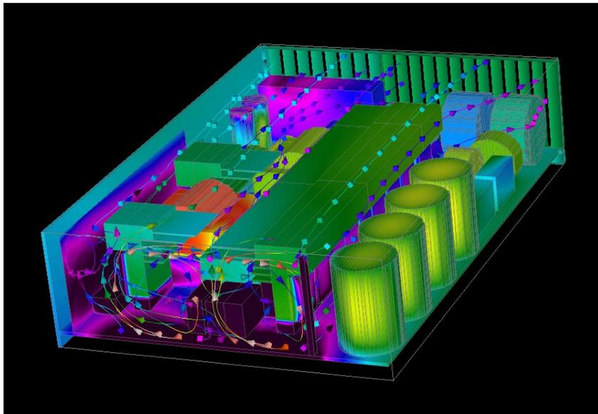
Coolit model of a rectifier unit.
