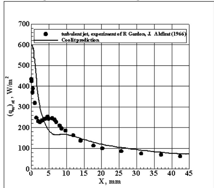
Left: Heat flux along the plate at  $Re=450$ . Right: Heat flux along the plate at  $Re= 2750$ .
