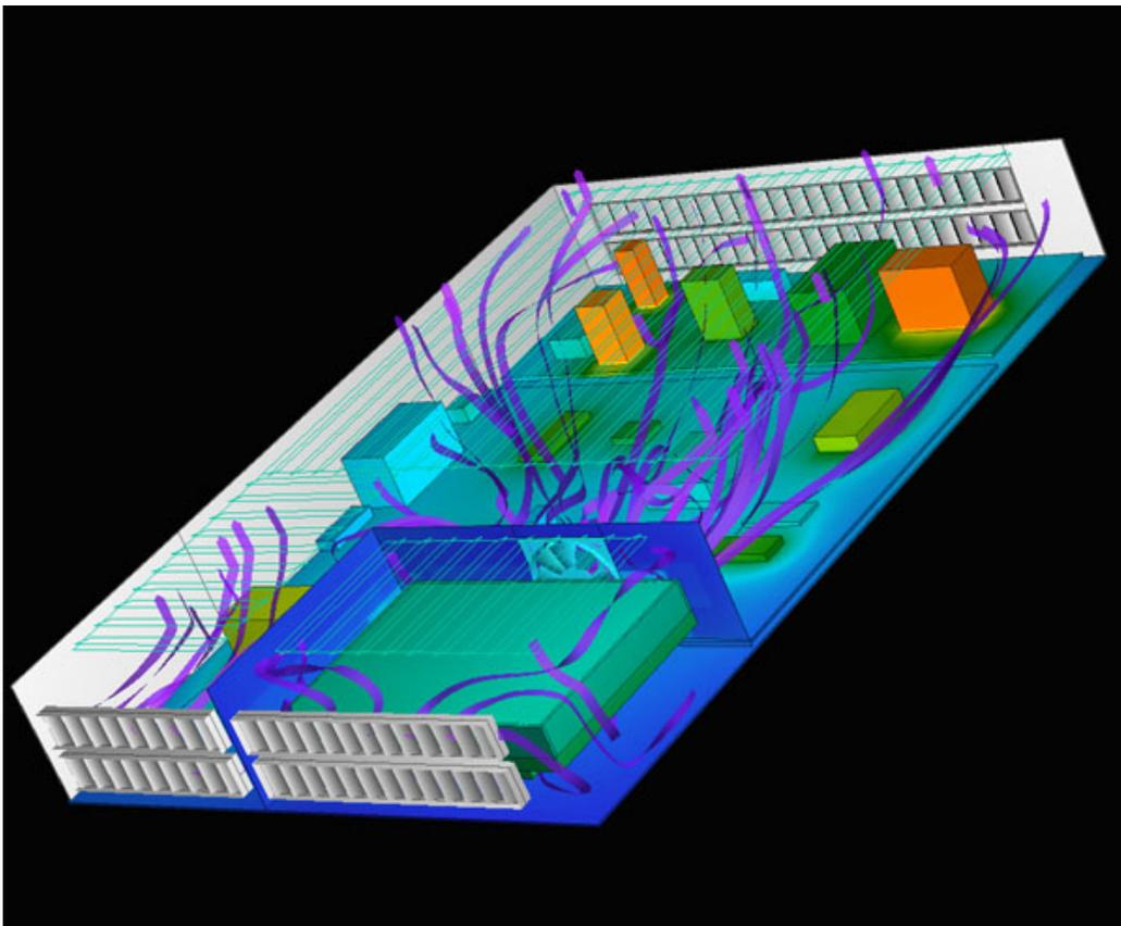
To maximize cooling efficiency while minimizing fan noise, the DVR fan is mounted on the divider wall surrounding the hard drive. Air drawn from the drive compartment passes through the divider wall to cool the electronics.
