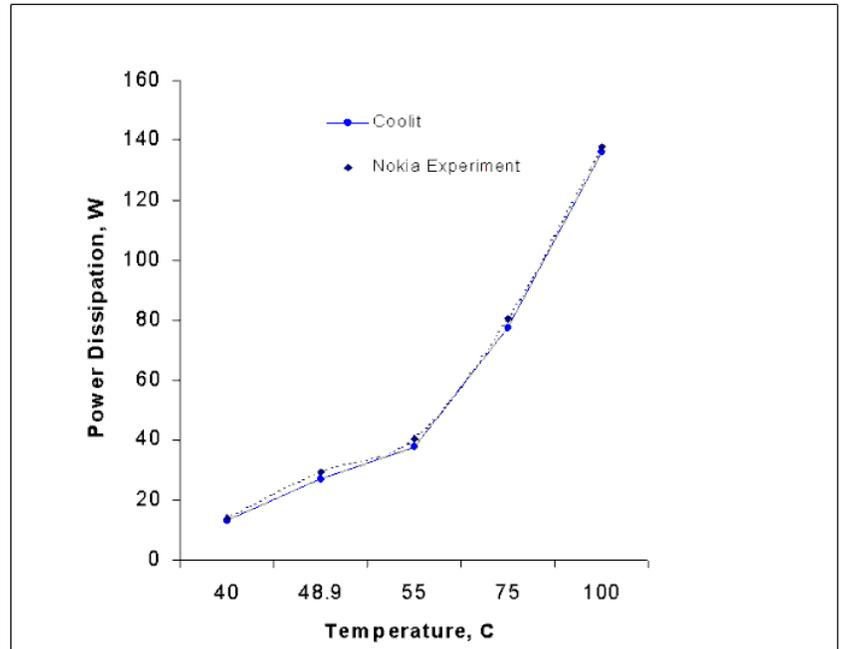
Flow pattern and predicted vs experiment power dissipation.
