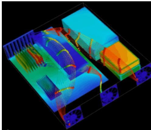
Redirecting more airflow towards the heat sink side of the assembly improved cooling.
