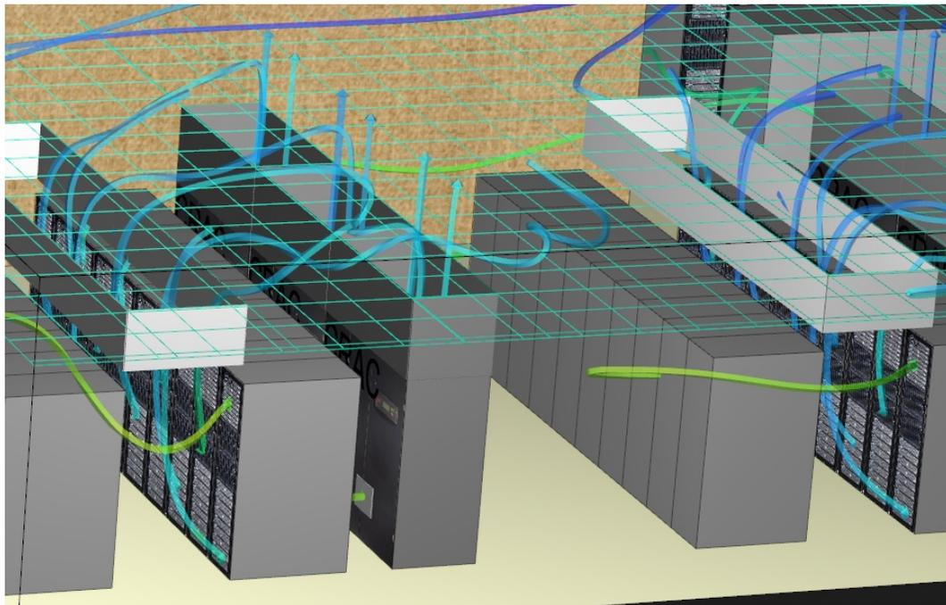
A portion of the IBM data center shows airflow using temperature-painted streamrods.
