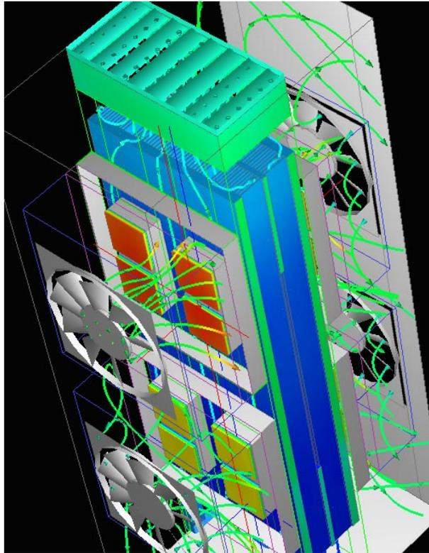
Coolit model of TEC-cooler for surgical blankets.
