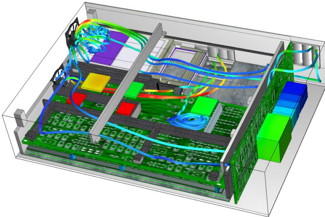
Coolit model of a Honeywell avionics system.
