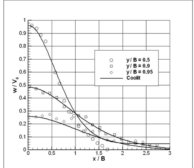
Fig 3. Velocity profile four jet-width from axis (left) and Fig. 4 shows y-velocity at several locations.
